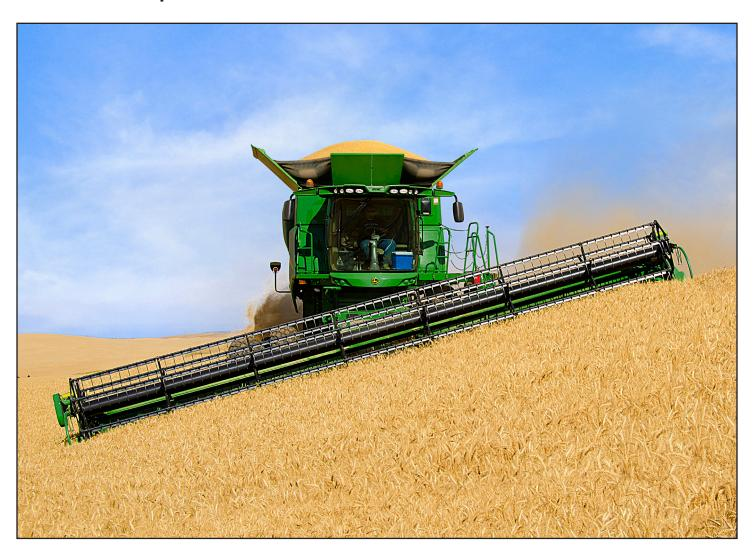
The Hillco Hillside Leveling System is designed for John Deere S Series combines. Hillco designed the Hillside Leveling System to maintain the combine's thrashing capacity and harvesting efficiency on contours of slopes up to 27%. This leveling system is designed to be installed with little modification to the combine.
