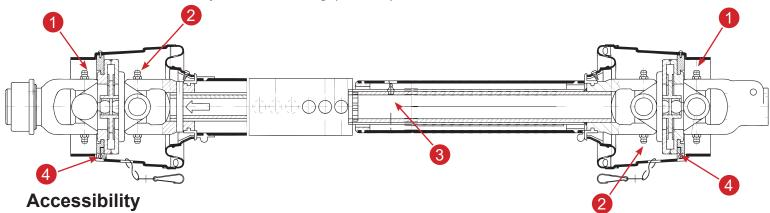
Each constant velocity driveline has at least 5 grease zerks (drivelines that have a stationary shield have at least 7 zerks). Due to various header/combine combinations some zerks may be inaccessible. Cutting a new hole in the profile shield is mandatory to access these zerks. Locate all zerks in your C.V. driveline and make sure there is access to properly grease each one. If the access hole is covered up due to the position of the driveline a new hole will need to be cut.
