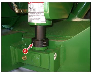
A - Mechanical Leveling Cylinder Stops (5/8" thick Cylinder Stops Shown)
