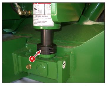
A - Mechanical Leveling Cylinder Stops 5/8 inch - Part # MC-137251 1/8 inch - Part # MC-137501
