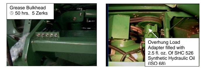
IMPORTANT! Recommended Oil Change Interval for the Over-Hung Load Adapter is 1000 Hrs. Please order Part Number LA-260401 for 2.5 fl. oz. of replacement oil. <u>Do Not Over or Under fill</u> or Damage to the Over-Hung Load Adapter may occur.
