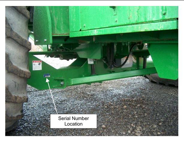
Write the serial number and the model number of the Leveling System on the lines provided. If needed, give these numbers to your dealer when you need parts or information for your Leveling System.
