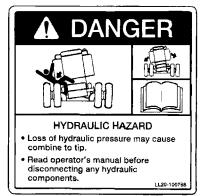
Label #4 Part number: LL20-100788 Locations: 3 (main cylinders and above leveling manifold)
