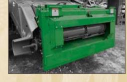
**CROP FEEDING SYSTEM**—The Sidehill header transition extends the feeder chain and provides feeding in all crops and conditions.
