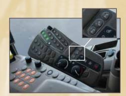
**LEVELING CONTROLS**—The leveling system controls are conveniently located in the John Deere CommandTouch™ Armrest Console. Select Automatic mode and the leveling system corrects for slope changes without any operator input. Switch to Manual mode and the Automatic leveling function is disabled, allowing the operator to have full control of the combine's chassis position.
