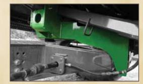
**REAR DROP AXLE**—The drop axle lifts the rear of the combine to match the 7" height increase of the overcarriage/undercarriage. This levels the combine fore/aft and accommodates both powered and non-powered rear axles.
