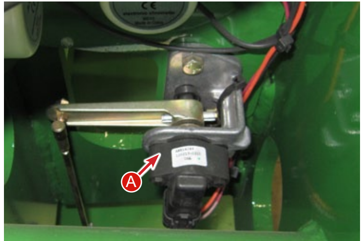
A - Overcarriage Position Sensor
