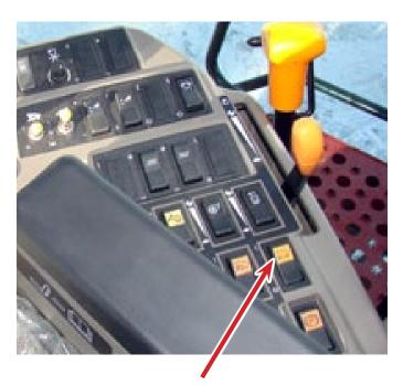
Rear Wheel Assist Engage/Disengage
