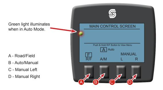
**Remote Leveling Switches:** Located on the armwrest control panel. These switches allow for Auto/Manual control and Left/Right leveling.
