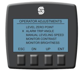
Once in the Alarm Trip Angle Page push and hold the ENT button for one (1) second to set the Alarm Trip Angle. This is a one (1) time adjustment unless tire size increases/decreases or the clinometer is replaced. Push ESC to leave the page.
