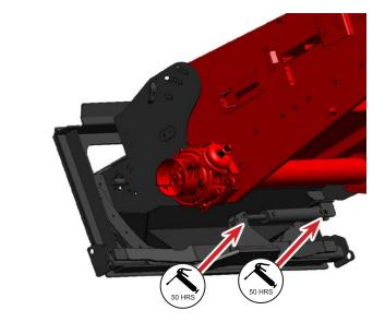
Slave Cylinder (base and rod ends) 50 hrs. 2 Zerks
