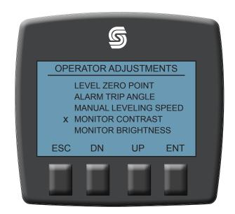
Once in the Monitor Contrast Screen, push the UP or DN buttons to increase or decrease the contrast (Default Setting is -3). Once the desired setting is reached, push and hold the ENT button for 1 second. This will lock the new monitor contrast setting. When done push the ESC button to leave the page.
