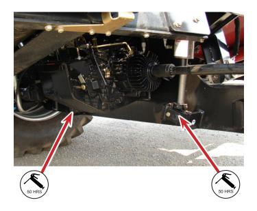
Transition Slip Clutch Grease on 50 hour interval with little to no slippage. Grease daily in adverse feeding conditions where slippage may occur more often. Pump until grease comes out.
