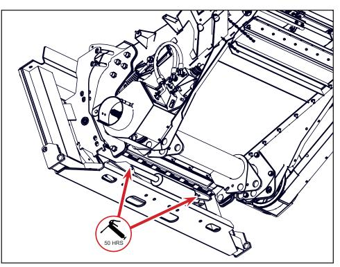
Slave Cylinder (base and rod ends) Below Feeder House 50 hrs. 2 Zerks
