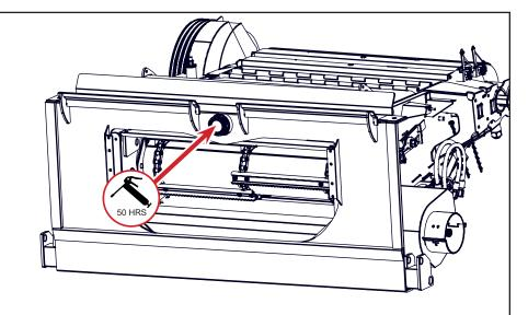
Transition Pivot Pin 50 hrs. 1 Zerks
