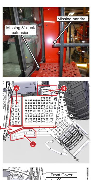
With certain tire sizes the latch (A) that locks the ladder in place may come in contact with the tires. If this occurs cut the handle off and reweld it so that it clears the tire.
