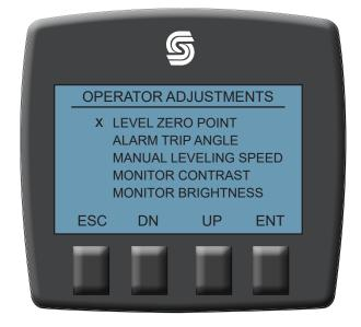
Once in the Level Zero Point Screen place a level on the cab floor. Manually level the combine to the left (L) or right (R) until the bubble shows level. Push and hold the ENT button for 1 second. This will set the Zero Point for Leveling. This is a one (1) time adjustment unless the clinometer or controller has been replaced. When done push the ESC button to leave the page.
