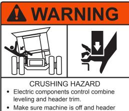
Make sure machine is off and header lock is down before making any adjustments to the electrical system.
