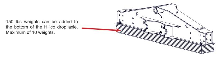
Use caution when using individual turning brakes. Installation of a Hillco Leveling System transmits additional weight to the rear axle of the combine. Excessive braking to turn can damage your combine chassis.
