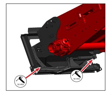
Slave Cylinder (base and rod ends) 50 hrs. 2 Zerks
