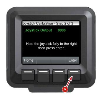
Push the Joystick lever all the way to the right and then press the Enter button (B).
