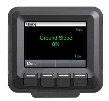
Push the up or down arrows to move to the desired function. Once the desired function is highlighted press the Enter button to go into that page. Press the Home button to go to the Home screen.
