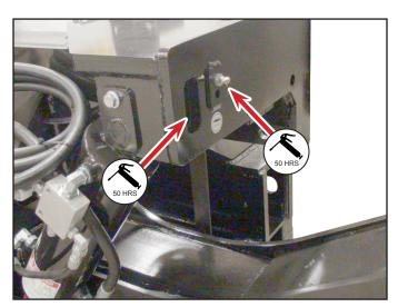
Master Cylinder (Base and Rod) 50 hrs. 2 Zerks
