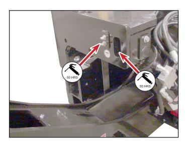
Leveling Cylinders Rod End 50 hrs. 2 Zerks
