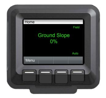
Push the up or down arrows to move to the desired function. Once the desired function is highlighted press the Enter button to go into that page. Press the Home button to go to the Home screen.
