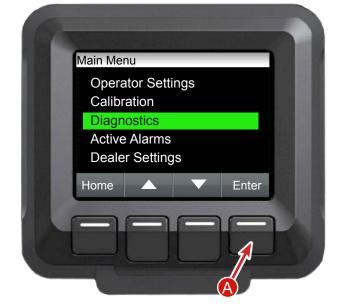
The Diagnostics menu allows the operator to view output information from the electrical system on the leveling system.
