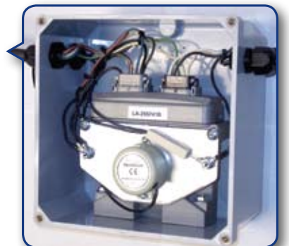
Clinometer and Controller
