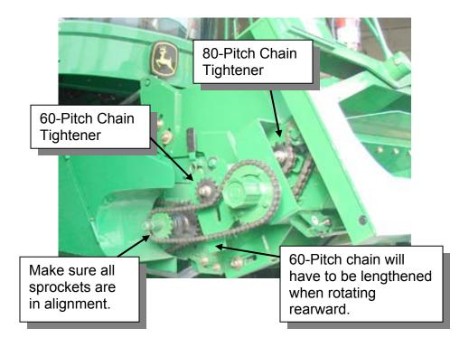
Do not over tighten these sprockets or premature chain and sprocket wear will occur.
