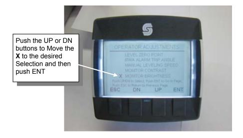
Once in the Level Zero Point Screen place a level on the cab floor. Manually level the combine to the left (**L**) or right (**R**) until the bubble shows level. Push and hold the **ENT** button for 1 second. This will set the Zero Point for Leveling. This is a one (1) time adjustment unless the clinometer or controller has been replaced. When done push the **ESC** button to leave the page. Note: Pushing the **ESC** button will take you back to the Menu Screen.
