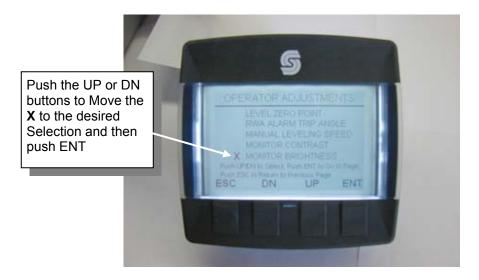
Once in the Monitor Brightness Screen, push the **UP** or **DN** buttons to increase or decrease the brightness (Default Setting is 8). Once the desired setting is reached, push and hold the **ENT** button for 1 second. This will lock the new monitor brightness setting. When done push the **ESC** button to leave the page. Note: Pushing the **ESC** button will take you back to the Menu Screen.
