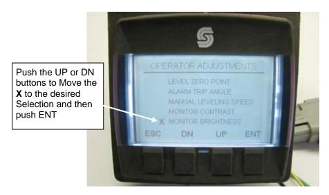
Once in the Alarm Trip Angle Page push and hold the **ENT** button for one (1) second to set the Alarm Trip Angle. This is a one (1) time adjustment unless tire size is changed. Push **ESC** to leave the page. Note: Pushing the **ESC** button will take you back to the Operator Adjustments Screen.
