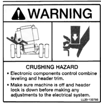
Label #5 Part number: LL20-100786 Locations: 1 (front of electrical box)
