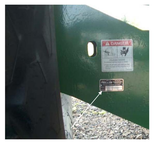
Write the serial number and the model number of the Leveling System and combine on the lines provided. It is important to reference these numbers when ordering parts or requesting technical support. It is suggested that you give the leveling system serial number to your John Deere dealer to be kept with their combine serial number records.
