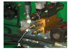
If the cycle time is shorter than the specification, turn the flow control set screw clockwise a quarter turn at a time until the cycle time meets the specification. If the cycle time is longer than the specification, turn the flow control screw counterclockwise a quarter turn at a time until the cycle time meets the specification.
