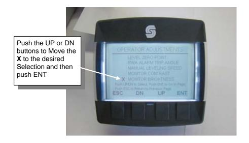
Once in the Alarm Trip Angle Page push and hold the **ENT** button for one (1) second to set the Alarm Trip Angle. This is a one (1) time adjustment unless tire size increases/decreases or the clinometer is replaced. Push **ESC** to leave the page. Note: Pushing the **ESC** button will take you back to the Operator Adjustments Screen.
