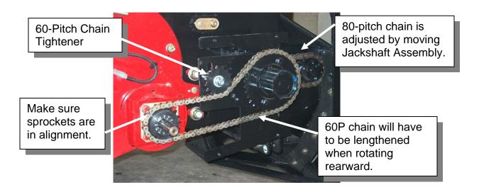
Do not over tighten idler sprockets or premature chain and sprocket wear will occur.
