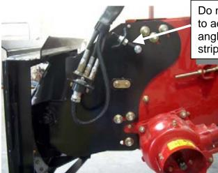
Do not use the eyebolt to adjust the header angle. The threads will strip.
