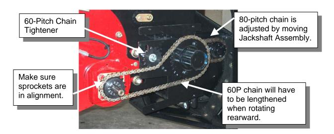
Do not over tighten these sprockets or premature chain and sprocket wear will occur.
