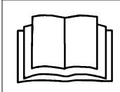
Decals, which display the "Read Operator's Manual" symbol, are intended to direct the operator to the Operator's Manual for further information regarding maintenance, adjustments and/or procedures for particular areas of the leveling system. When a decal displays this symbol refer to the Operator's Manual for further instructions.
