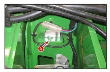
A - Slope Sensing Clinometer
