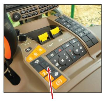
Rear Wheel Assist Engage/Disengage
