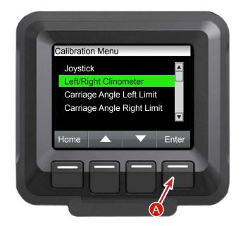
Follow the directions on the screen. When the combine is level side to side press Enter (A).
