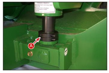
A - Mechanical Leveling Cylinder Stops (5/8" thick Cylinder Stops Shown)
