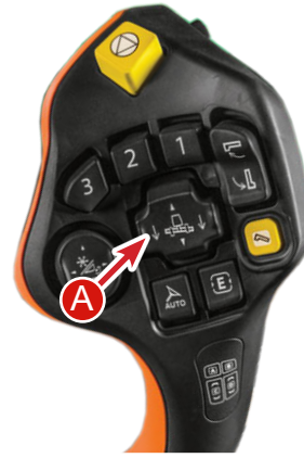
A - Header Trim Switch B - Master Cylinder
