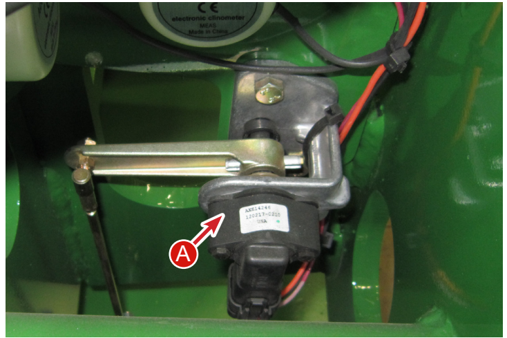
A - Undercarriage Position Indicator
