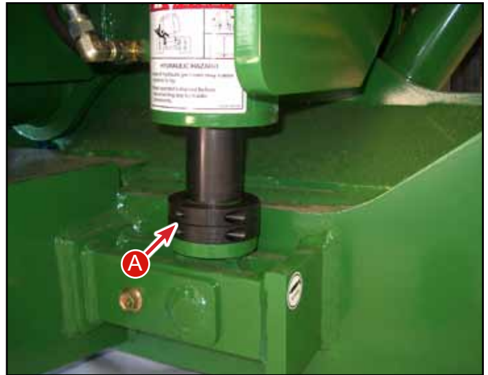
A - Mechanical Leveling Cylinder Stops (5/8" thick Cylinder Stops Shown)
