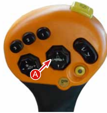
A - Header Trim Switch B - Master Cylinder
