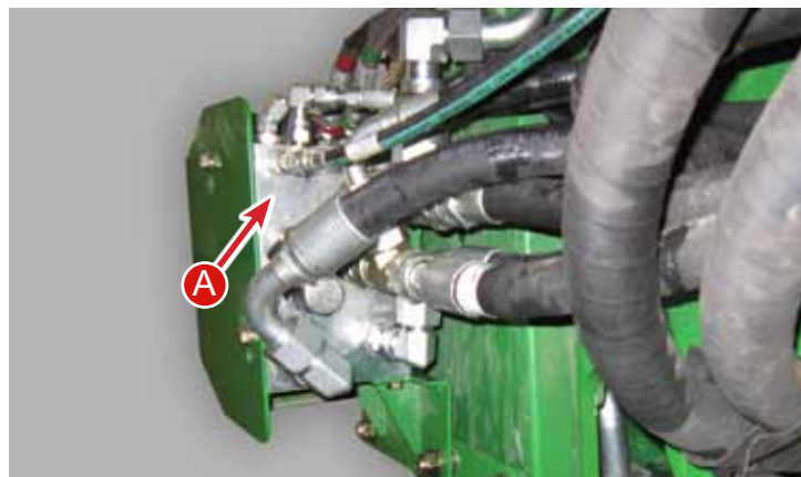
A - Header Height Valve Block
