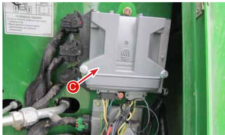
C - Leveling Controller
