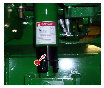
B - Cylinder Safety Stops C - Cylinder Safety Stop Holder
