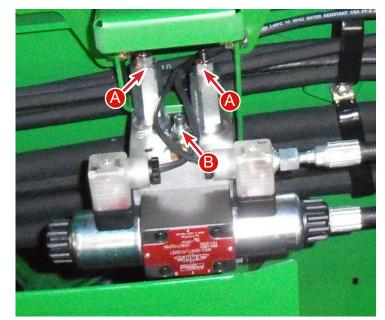
A - Trim Relief Valves B - Tilt Flow Control Valves
