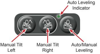
Auto/Manual Leveling— The Auto/Manual leveling button is used to toggle between the Automatic and Manual Modes. In Manual Mode the chassis will not rotate until initiated by the operator. In Automatic Mode, rotation of the chassis is initiated by the controller as dictated by changes in the slope. The operator can momentarily override the controller using the Manual Left and Right Buttons. The combine will return to level once the buttons are depressed.
