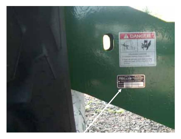
Write the serial number and the model number of the leveling system and combine on the lines provided. It is important to reference these numbers when ordering parts or requesting technical support. We suggest that you give the leveling system serial number to your John Deere dealer to be kept with their combine serial number records.
