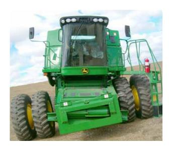
The Hillco Sidehill Leveling System is designed for John Deere STS combines. Hillco designed the Sidehill Leveling System to maintain the STS combine's thrashing capacity and harvesting efficiency on contours of slopes up to 18%. This leveling system is designed to be installed with little modification to the combine.
