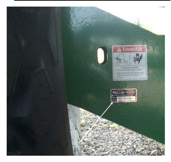
Write the serial number and the model number of the Leveling System and combine on the lines provided. It is important to reference these numbers when ordering parts or requesting technical support. We suggest that you give the leveling system serial number to your John Deere dealer to be kept with their combine serial number records.
