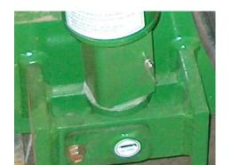
When the leveling cylinder safety stops are installed on the leveling cylinders, the carriage cannot rotate. The stops must be installed before working on or around the leveling system and also when hauling the combine. It is recommended that the stops during long term storage. When the stops are not being used, they should be stored on the mount next to the leveling cylinder.
